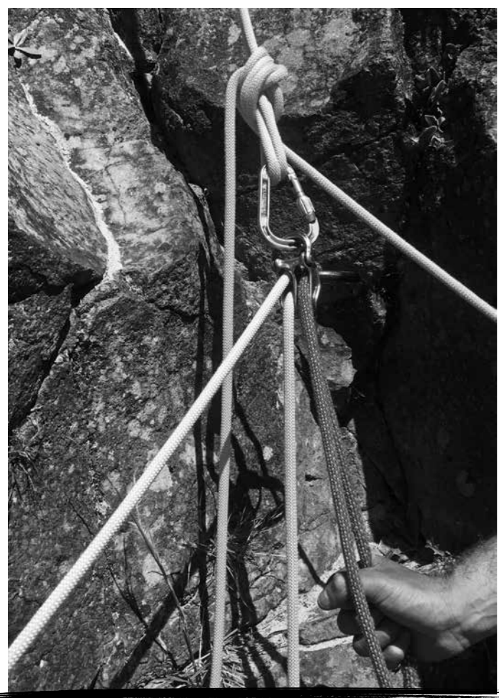
Reconstruction of the belay set up. The climber fell on the (orange) rope which is coming up diagonally from the left. The right hand (purple) rope was weighted, preventing the belay device from moving fully into line with the direction of force; the load side of the orange rope on top slid to the side of the belay device, rather than cinching down on the lower section of rope. The Pivot is presently in space, but was dragged onto the rock protrusion to the left when the climber fell.
