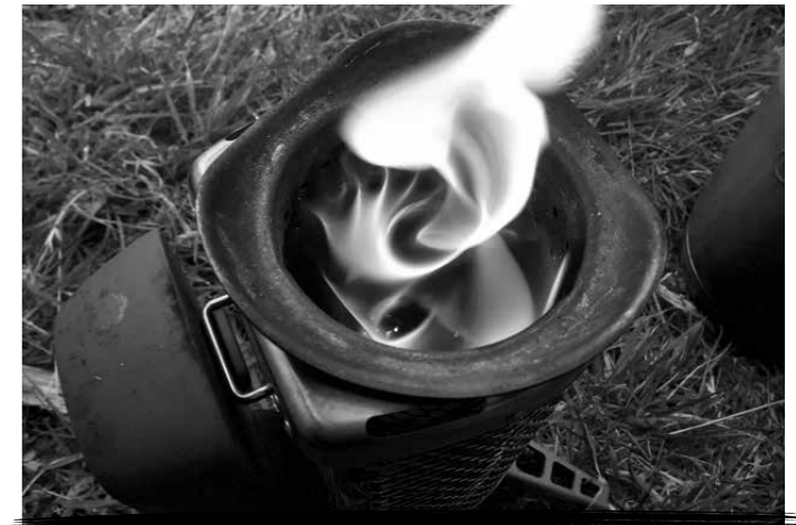
The gasifying effect generates a vortex like flame in the Biolite Cookstove. Cheaper to fuel than conventional stoves even if fuel is purchased.
