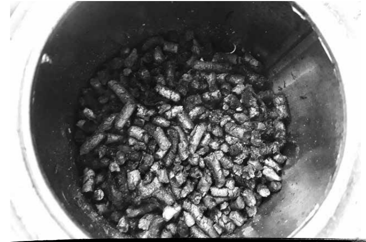
Cooled, stored & carried away in a sealed tin, charred wood-pellets make ideal biochar.
