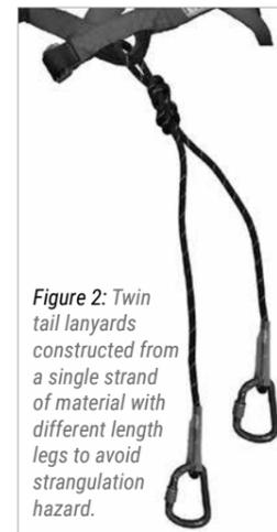
Figure 2: Twin tail lanyards constructed from a single strand of material with different length legs to avoid strangulation hazard.
