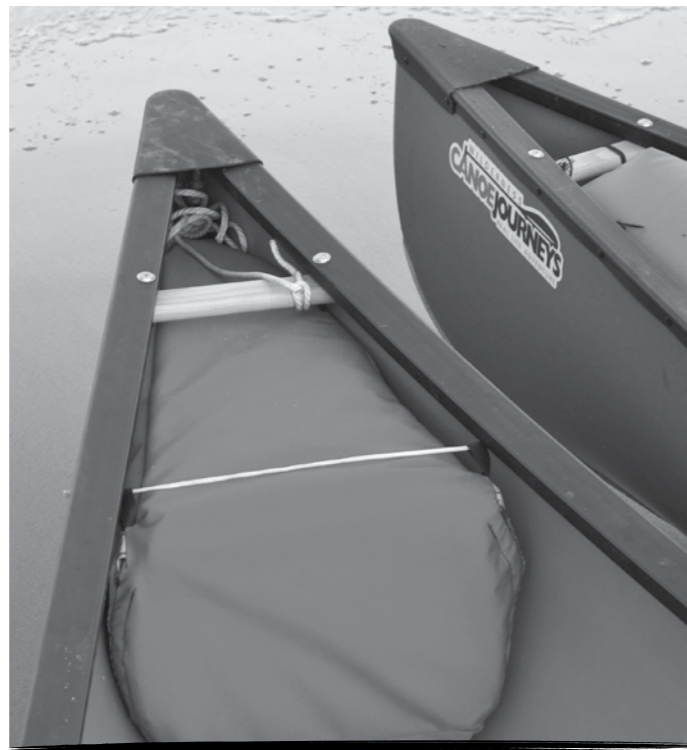
Solid foam buoyancy blocks
